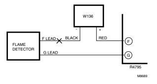
Insert a 117053 Meter Connector Plug, wired color-tocolor to the W136 leadwires, into the test jack on the amplifier (Fig. 10). This automatically puts the microammeter in series with the flame detector.
